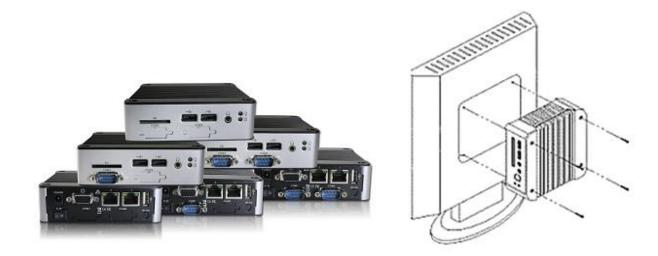
EBOX-336x Series is a revolutionary device especially designed for limited physical space and temperature concerns. No matter you are in a jammed office, a crowded place, or public transportation, EBOX-336x can be easily integrated with a VESA monitor to access at any time.
