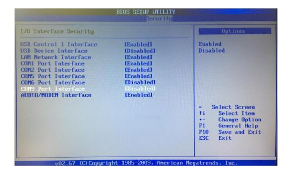
For user want to use mPCle via COM port signal, set BIOS COM9 Port Interface enabled as below: Move to **Security** → I/O Interface Security and set BIOS COM9 Port Interface as enabled. Press <F10> to save the setting and exit.
