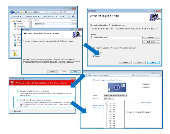
After VGA driver installed, restart the unit, user will be able to select the resolution up to 1920 x 1080 pixels.
